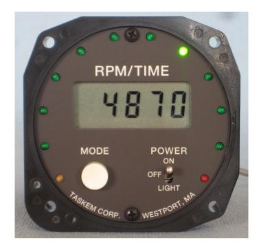
zero each time the engine is first started, thus it very closely represents current flight time and can be observed anytime during flight.
