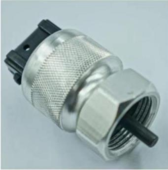
The Taskem Hall Effect sender is compatible with the mechanical tachometer port on Lycoming, Continental and many other popular aircraft engines. For these it is the ideal companion to our Model 4000 tachometer. It is not dependent on magnetos so RPM is always displayed regardless of shutting either mag off during run up. This combination is so sensitive and stable that a noticeable difference in top RPM can be seen during run up when facing into or away from the wind.
