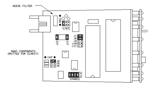
Jumpers J1, J2 or J3 select the SENSITIVITY of the input circuit, which is a measure of the magnitude of the electrical signal required by the tach. In general, J1 is used when the peak voltage of the input signal is between 3 and 20V, J2 for 10-60V and J3 for 30-200V. Usually, only one jumper is installed. There is also the option to install no jumpers and solder a custom sensitivity resistor in the holes labeled RES.
