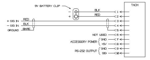
The electrical diagram above shows the function of all wires. Take a moment to examine the connector that was just removed. You will see the 9V battery clip at one end. The black wire going to the battery clip is pin/wire #1 and every wire thereafter is numbered sequentially through #10. A shielded cable is connected to pins 3, 4 & 5. The red cable wire is the positive signal input and the black is negative. There is also bare shield wire that might need to be
